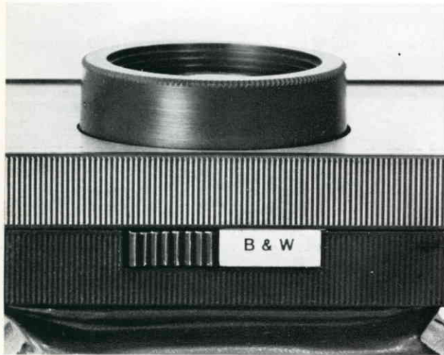
Set the Film Selector as shown for black and white pictures with 3000 speed film.
